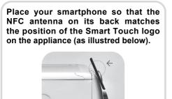
If you do not know the position of your NFC antenna, slightly move the smartphone in a circular motion over the Smart Touch logo until the App confirms the connection. In order for the data transfer to be successful, it is essential TO KEEP THE SMARTPHONE ON THE DASHBOARD DURING THESE FEW SECONDS OF THE PROCEDURE; a message on the device will inform about the correct outcome of the operation and advise you when it is possible to move the smartphone away.
